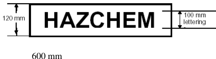
Figure 13.1 Form and dimensions of outer warning placard
