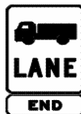
End truck lane sign
