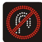
No U-turn sign (Variable illuminated message sign)
