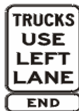
End trucks use left lane sign
