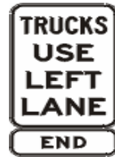
End trucks use left lane sign
