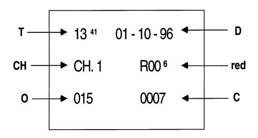
T is the time, in 24-hour clock mode, when the image was captured.
