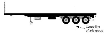
converter dolly means a trailer with a single axle or 1 axle group, and a fifth wheel coupling, designed to convert a semitrailer into a dog trailer.
