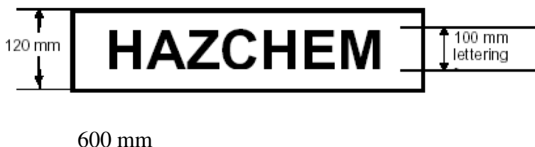
Figure 13.1 Form and dimensions of outer warning placard
