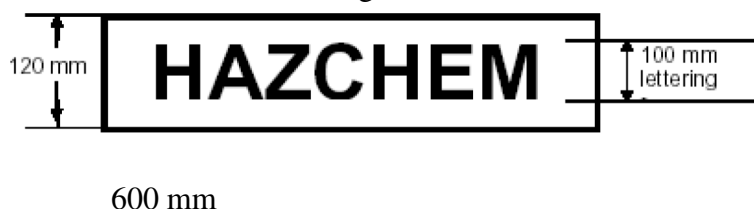
Figure 13.1 Form and dimensions of outer warning placard
