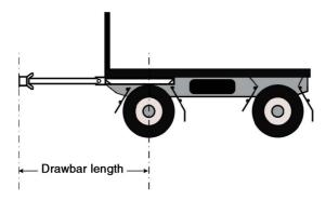
(2) For a trailer with 1 axle group or a single axle, other than a semitrailer, the distance between the pivot point of the coupling on a drawbar of the trailer and the centre line of the trailer's axle group or single axle must not be more than 8.5m.
