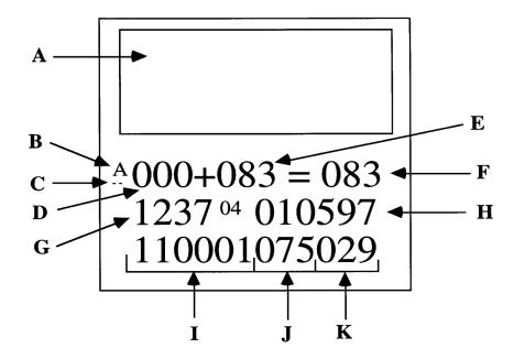
A is details written by the operator of the system's camera, when a film magazine is inserted, that are superimposed on each image on the film as it is captured.
