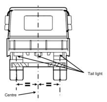
(4) Tail lights fitted to a vehicle in accordance with this division may also serve as rear clearance lights if the tail lights are fitted to the vehicle in accordance with section 89(3).
