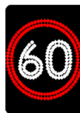
Speed limit sign (Variable illuminated message sign)
