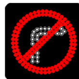
No right turn sign (Variable illuminated message sign)
