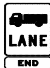
End truck lane sign
