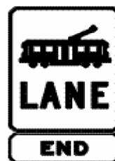
End tram lane sign
