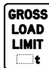
Gross load limit sign
