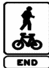
End shared path sign
