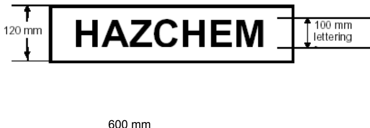
Figure 13.1 Form and dimensions of outer warning placard
