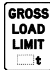
Gross load limit sign
