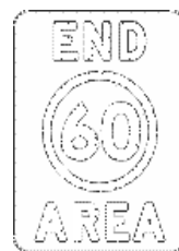
End area speed limit sign
