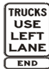
End trucks use left lane sign
