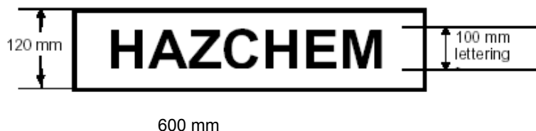
Figure 13.1 Form and dimensions of outer warning placard
