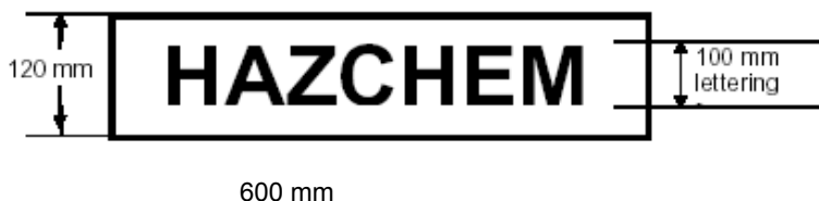
Figure 13.1 Form and dimensions of outer warning placard
