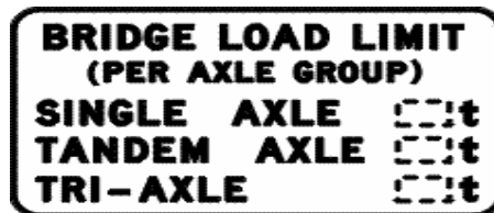
Bridge load limit (mass per axle group) sign
