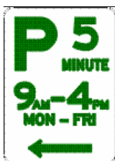
Example 3 Permissive parking sign with a number of minutes to the right of P
