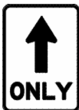
No turns sign
