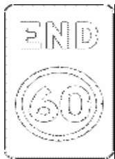
End speed limit sign
