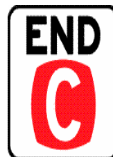
End clearway signs
