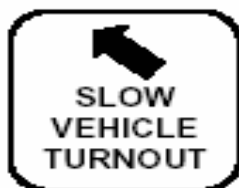
Slow vehicle turn out lane sign
