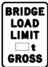
Bridge load limit (gross mass) sign
