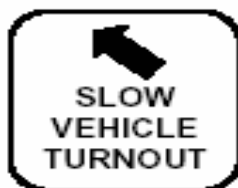
Slow vehicle turn out lane sign
