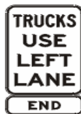
End trucks use left lane sign
