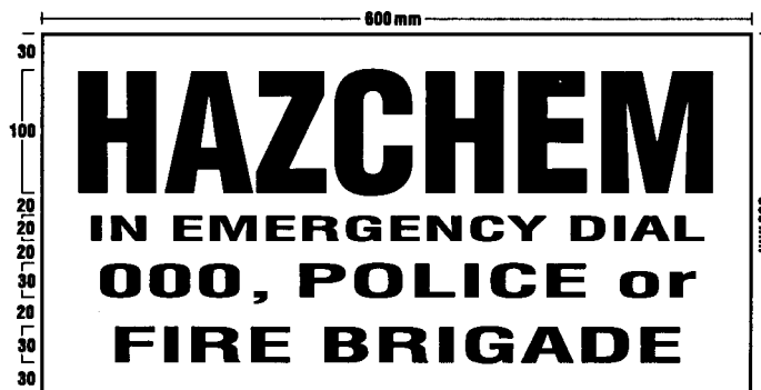
figure 2—outer warning sign
