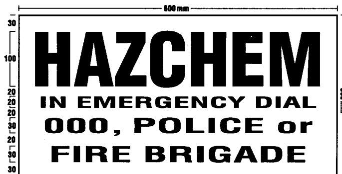
figure 2—outer warning sign
