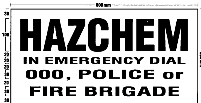
figure 2—outer warning sign
