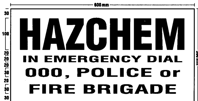
figure 2—outer warning sign
