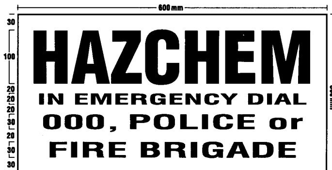
figure 2—outer warning sign
