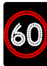
Speed limit sign (Variable illuminated message sign)
