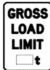
Gross load limit sign
