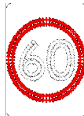
Speed limit sign (Variable illuminated message sign)
