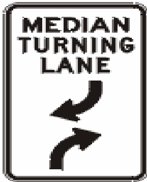
Example 1 Median turning lane sign
