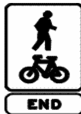
End shared path sign
