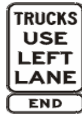
End trucks use left lane sign
