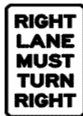
Right lane must turn right sign
