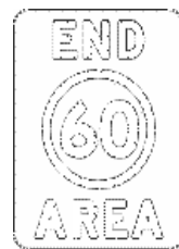
End area speed limit sign
