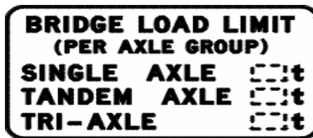
Bridge load limit (mass per axle group) sign
