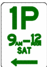
Example 1 Permissive parking sign applying to a length of road with a whole number to the left of P
