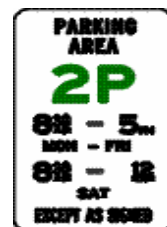
Example 2 Permissive parking sign applying to an area with a whole number to the left of P
