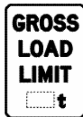
Gross load limit sign
