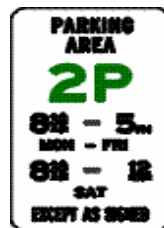
Example 2 Permissive parking sign applying to an area with a whole number to the left of P
