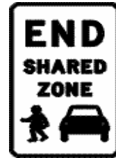
End shared zone sign
