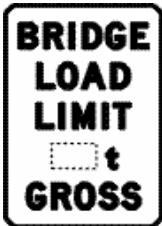
Bridge load limit (gross mass) sign
