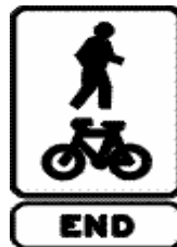
End shared path sign
