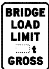
Bridge load limit (gross mass) sign
