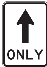
No turns sign
