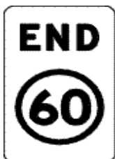
End speed limit sign
