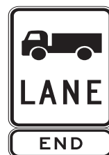
End truck lane sign
