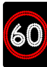
Speed limit sign (Variable illuminated message sign)
