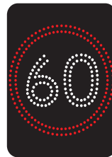
Speed limit sign (Variable illuminated message sign)
