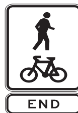
End shared path sign
