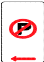
No parking sign (for a length of road)
