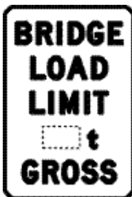
Bridge load limit (gross mass) sign
