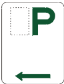
Permissive parking sign (for a length of road)
