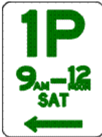
Example 1 Permissive parking sign applying to a length of road with a whole number to the left of P
