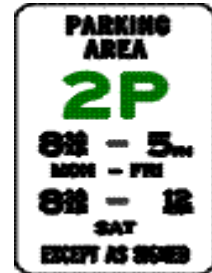
Example 2 Permissive parking sign applying to an area with a whole number to the left of P
